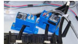
The WA-118 model also includes the capability to measure the temperature of an included Type-K thermocouple from -18C to +105C (0F to 220F.) In many instances, our customers have found that power consumption can be linked to temperature issues - internal and/or external temperature fluctuation. The inclusion of a Type-K thermocouple electrical interface and sensor provides the capability to monitor temperature while the electrical power is being monitored.
