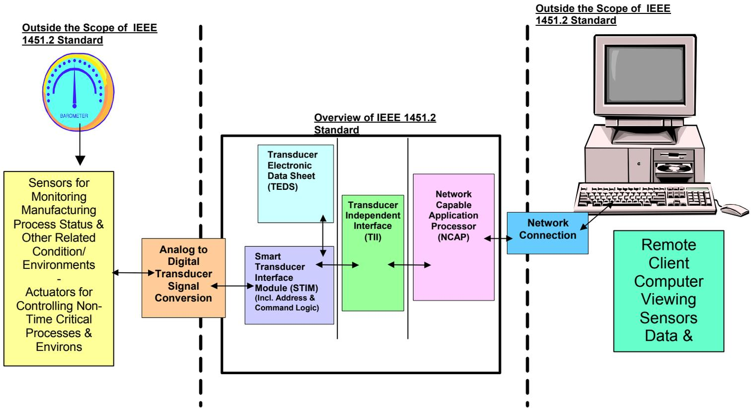
Figure 2. A Network Enabled Equipment Monitor Using IEEE 1451.2 technology to accommodate multiple types of “equipment-status indicating” transducers
